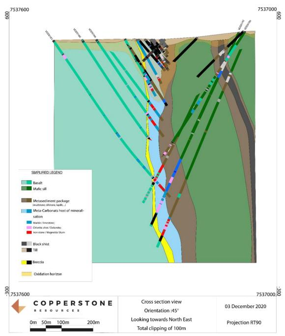
Figure 8.4. Detailed cross section across the D zone.
