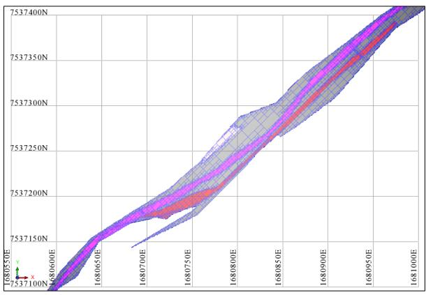
Figure 9.16. Plan view of the Viscaria D zone at elevation 0mRL which is about 500 metres below surface. Orientation of the rotated block model vs magnetite skarn shape (yellowish gray), D1 mineralisation (purple) and D2 mineralisation (red).
