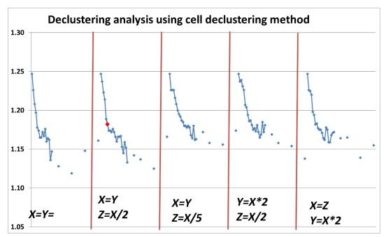
Figure 9.7. Declustering analysis to test impact of sample clusters to the mean grade. Domain 101.
