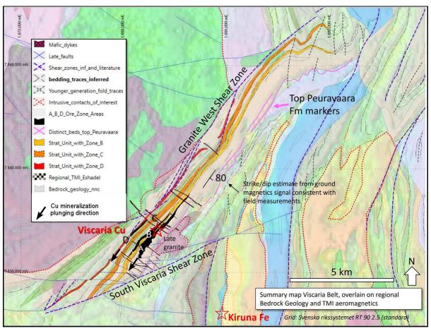
Figure 8.2. The South Viscaria shear zone controls the south extension of the ore hosting lithologies. Drilling intersections and structural interpretations Pratt, 2020 for extension of the D ore lenses at depth indicates partly an structural control on the steeply dipping plunge of higher Cu grades and increased mineralized thickness towards the South West.
