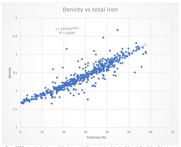
Figure 9.23 Scatter plot showing correlation between total iron content and density of the rock. Correlation of density to iron is exceleint, allowing polynomial fitting as a comparative density calculation method.
