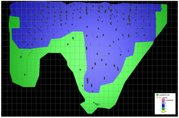
Figure 9.29. Longitudinal view showing resource classification and composites in the estimation. Blue colour shows indicated resources and green colour shows inferred resources. Black dots are sample composites used in the estimation.
