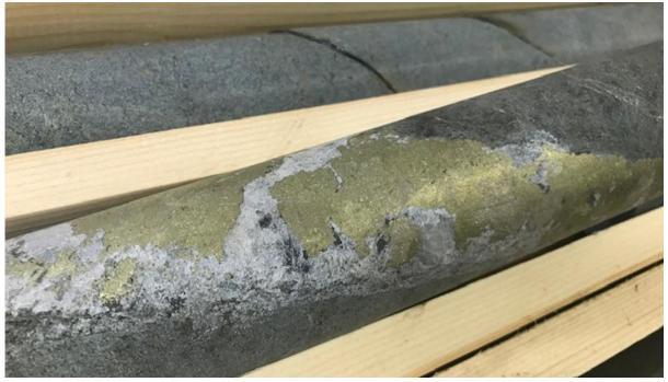
Figure 8.6. Chalcopyrite carbonate vein cuts through coherent intrusive units located on the hanging wall side of the D lens.
