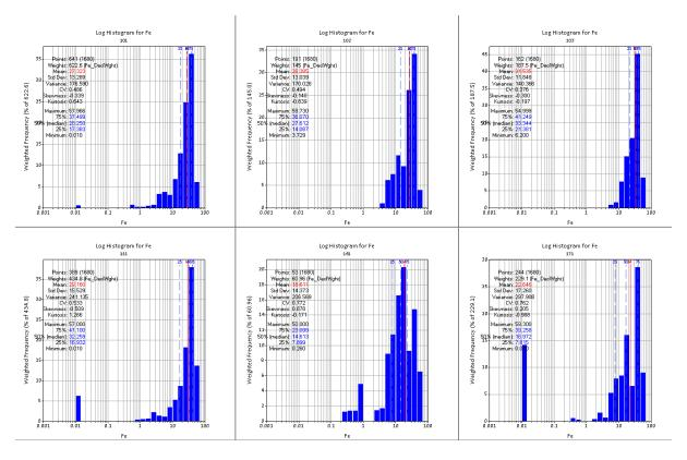
Figure 9.10. Iron grade population in the log histogram. X-axis shows iron grade and y axis shows frequency. Domains from left to right are top row 101, 102, 103 and bottom row 111, 161, 171.
