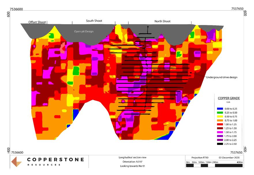
Figure 9.18. SW-NE longitudinal section over D zone showing estimated copper grade in the block model with 2016 scoping study mine design shapes
