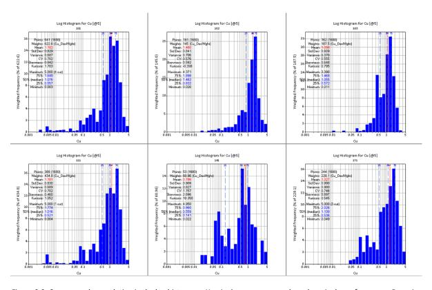
Figure 9.9. Copper grade population in the log histogram. X-axis shows copper grade and y axis shows frequency. Domains from left to right are top row 101, 102, 103 and bottom row 111, 161, 171.
