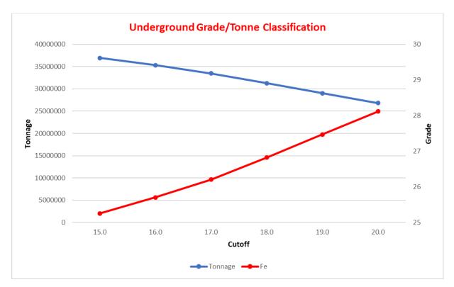
Figure 9.35. Grade tonnage curve of underground mineral resources of all fe domains.
