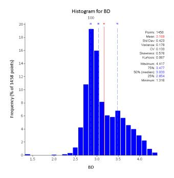
Figure 9.22. Bulk density of the magnetite skarn of Viscaria D zone.
