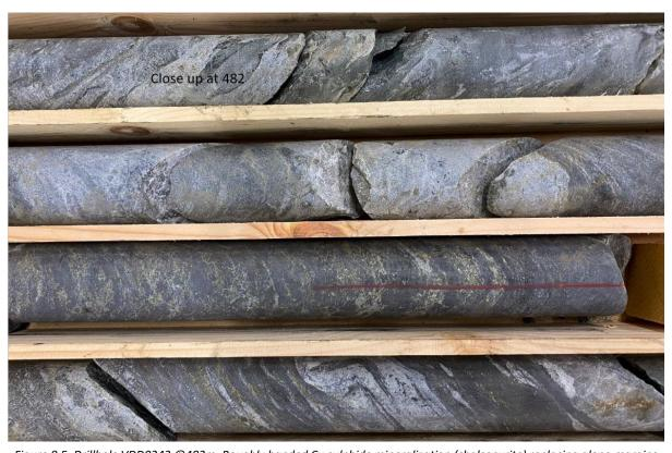
Figure 8.5. Drillhole VDD0242 @482m. Roughly banded Cu sulphide mineralization (chalcopyrite) replacing along margins of magnetite zones and disseminated carbonates in the D ore.
