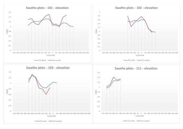
Figure 9.26. Swath plots Cu(%) vs elevations showing sample grades in red and model grades in blue.
