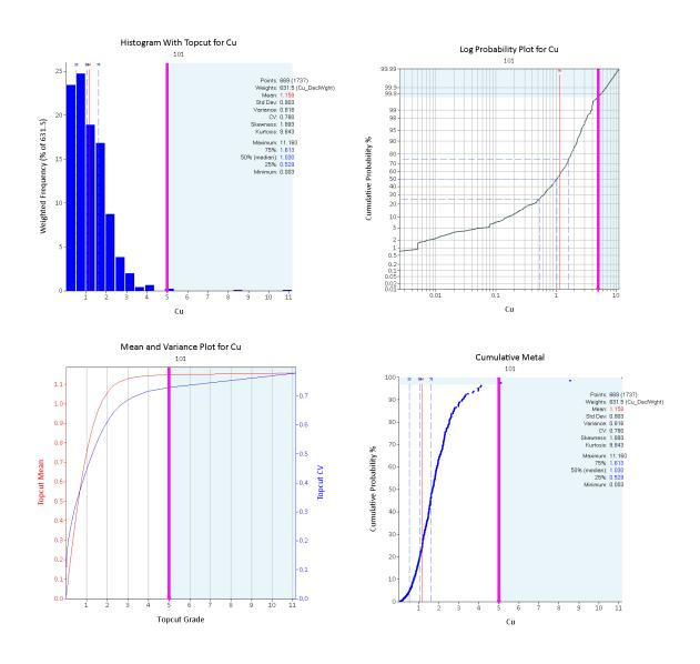
Figure 9.8. Topcut analysis using continuity and tail of the histogram (top left), change of the slope in the log-probability plot (top right), mean-variance plot (bottom left) and cumulative metal (bottom right).
