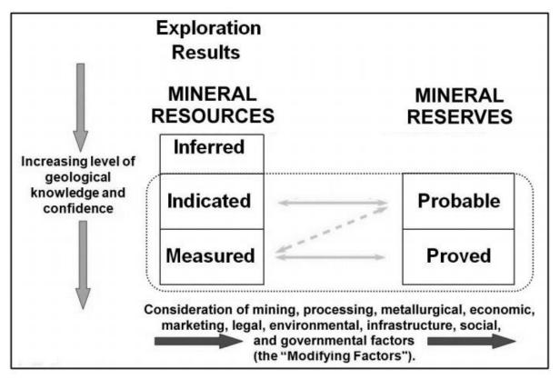
Figure 9.28. PERC standard guideline for resource classification.
