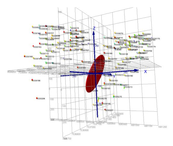
Figure 9.12 Image shows variogram ellipsoid for Cu and composite sample data in the domain 101.
