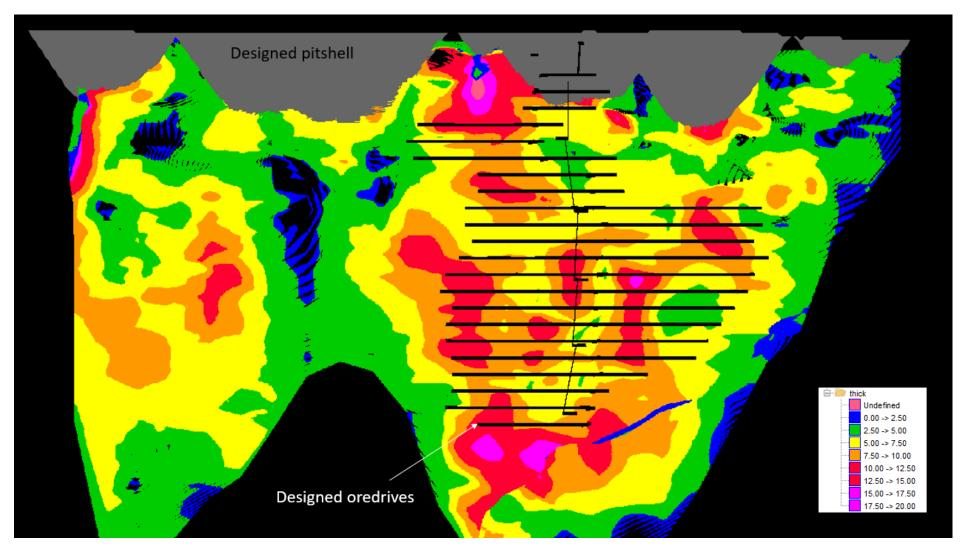
Figure 9.19 SW-NE longitudinal section with thickness variations in the D1 mineralisation with 2016 scoping study's mine design shapes.
