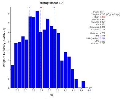
Figure 9.21. Bulk density of the copper mineralisations of Viscaria D zone.
