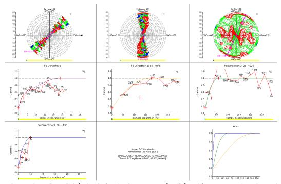
Figure 9.14. Variography analysis for iron in domain 101. Images are from left to right: top row. Variance images in the strike plane (left), dip plane (middle) and plunge plane (right). Center. Directional variograms major direction (left), semimajor direction (center) and minor direction (right). Bottom. True downhole variogram (left), modelled direction definition (center) and modelled variograms in normal score space (right).
