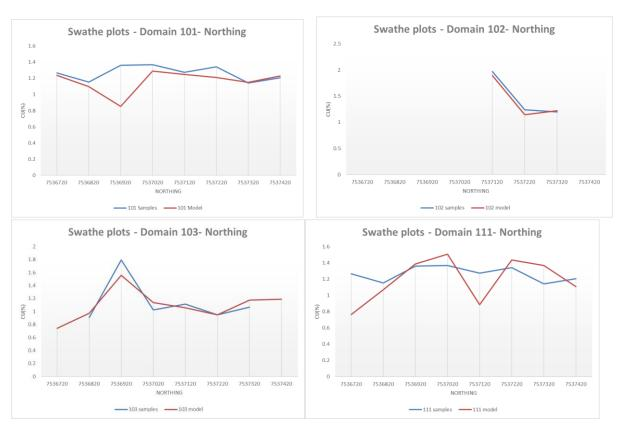
Figure 9.25. Swathe plots Cu(%) vs northing showing sample grades in blue and model grades in red.
