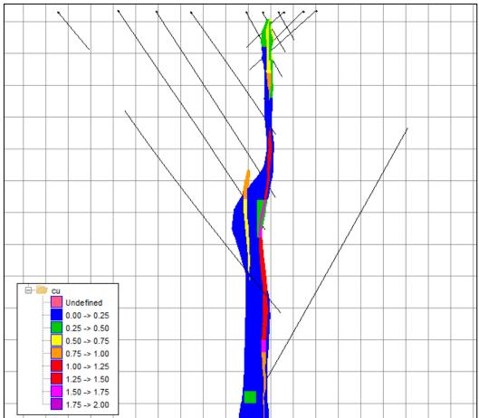
Figure 9.17 shows an example of the final block model after ordinary kriged estimation. Image shows profile in the D zone south. Estimated block model grades are shown in filled shapes which is coloured by copper grade
