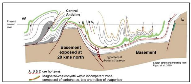
Figure 5.2. Schematic representation of deformation style recognized in the Finnish part of comparable Paleoproterozoic greenstone mafic sedimentary sequences overlying the Archean basement. A, B and D Viscaria ore horizons are tentatively marked in this adapted sketch as to enhance the role of basement structures in the Viscaria area.
