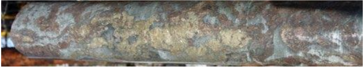
Figure 12-1: Drillcore from the Eva deposit at 400m depth, outside the mineral resource boundary.
