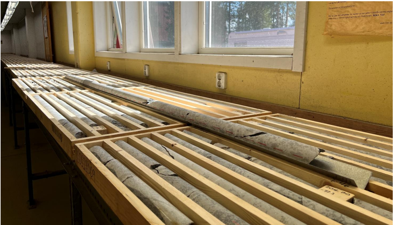
Figure 8-2: Photograph from the SGU logging facility in Malå, with drill core from twin hole COS22009 displayed on the tables. Orientation marks were being drawn onto the core.
